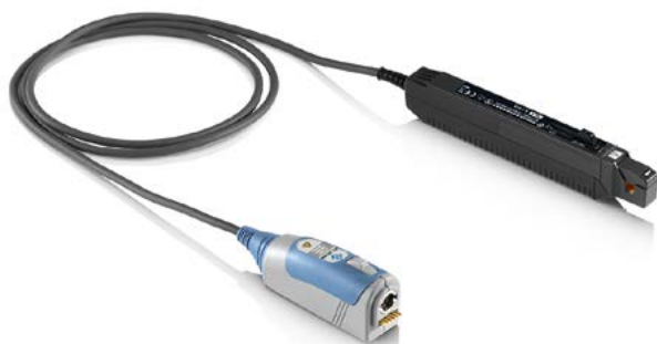
R&S®RT-ZC20B current probe (100 MHz, 30 A (RMS)).
