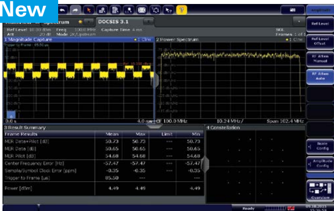
Analysis of DOCSIS 3.1 upstream signal with option R&S®FSW-K193.
