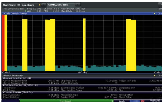
Demodulation of a CDMA2000® base station signal with R&S®FSW-K82.
