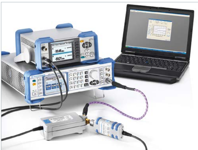
Calibration of an R&S®NRP-Z55 thermal power sensor.
