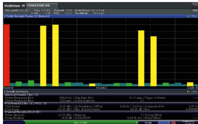
Demodulation of a CDMA2000® mobile station signal with R&S®FSW-K83.
