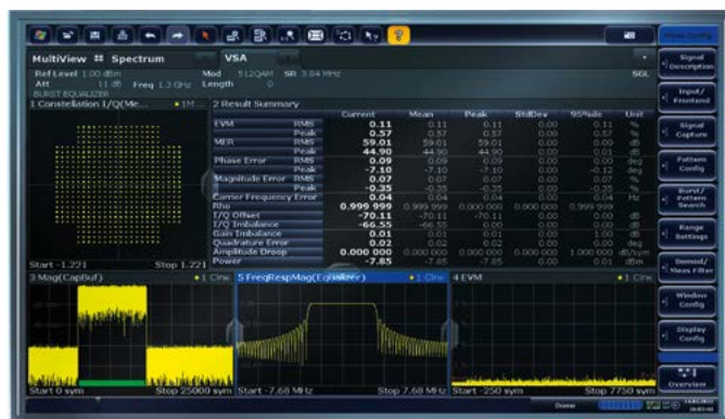
Demodulation of a 512QAM signal with R&S®FSW-K70.
