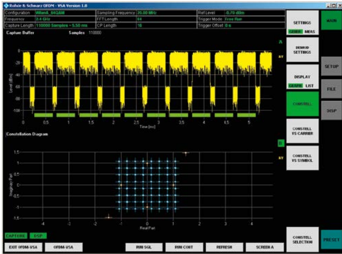
The upper part of the display shows the recorded signal in the time domain. The lower part shows the constellation diagram.
