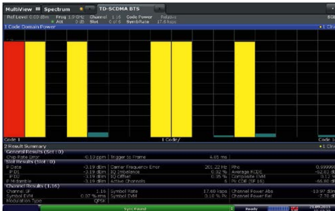
Demodulation of a TD-SCDMA base station signal with R&S®FSW-K76.
